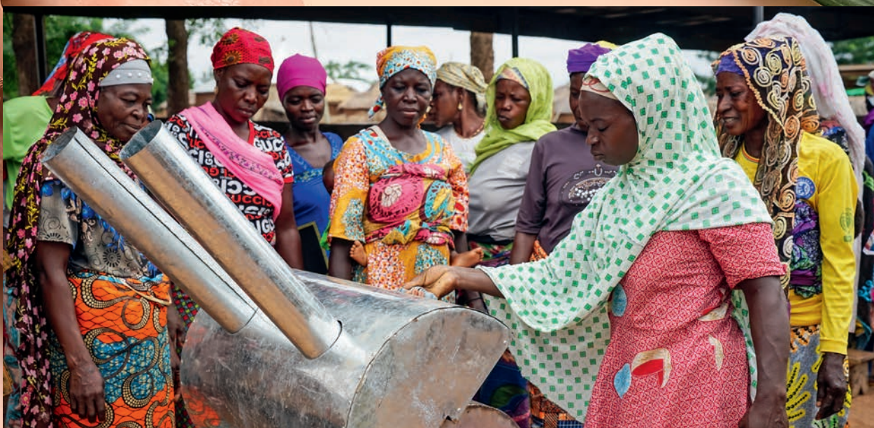
These new shea nut roasters can primarily use shea cake for fuel, reducing the reliance on firewood.
